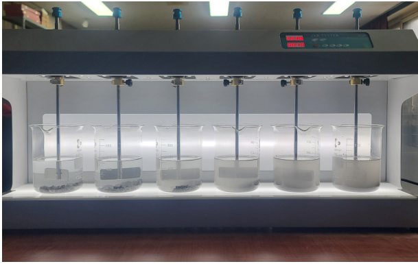
Fig. 2. Jar-Test by steel slag particle size
